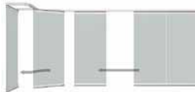
Sliding the panels towards the opening side
