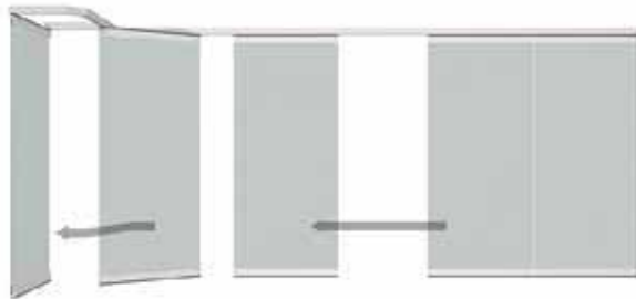
Sliding the panels towards the opening side
